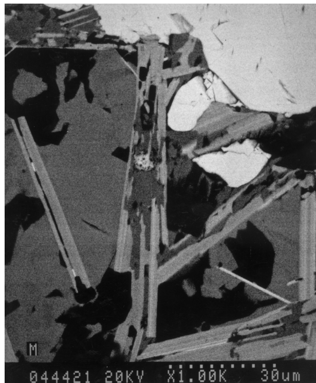
Figure 2: Backscattered electron image showing relic of burbankite in platy crystal of synchysite (centre of image), strontianite (gray) and baryte (white).
